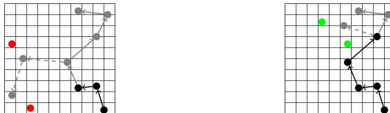
Figure 4-7: Left: long processing may cause large gaps between new routes calculated by the driver (solid gray) and the outdated ones stored at the scheduler (dashed gray), yielding bad matches (red dots). Right: with short processing, the matched requests are close to the actual routes (green dots).
